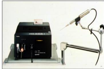
Polarographic oxygen (Eppendorf) electrodes
